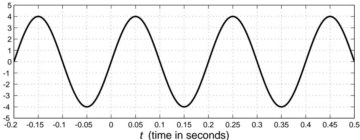
The above graph is a plot of a sinusoidal signal  $x(t) = A \cos(\omega_0 t + \phi)$ .
