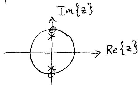
This IIR filter is stable, and it provides nulling at  $\hat{\omega} = \pm \frac{\pi}{2}$  or, since  $f_s = 1000$  samples/s, at  $\omega = \hat{\omega}f_s = \pm 500\pi$  rad/s.
