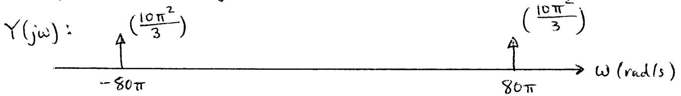
$$Y(j\omega) = \frac{10\pi^2}{3} \left( \delta(\omega+80\pi) + \delta(\omega-80\pi) \right)$$
