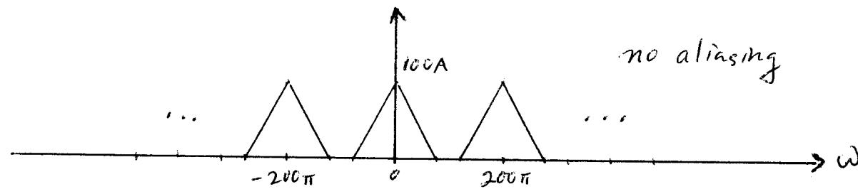
(c) using sampling frequency from part (b)  $\Rightarrow X_R(j\omega) = H_R(j\omega)X_s(j\omega)$
