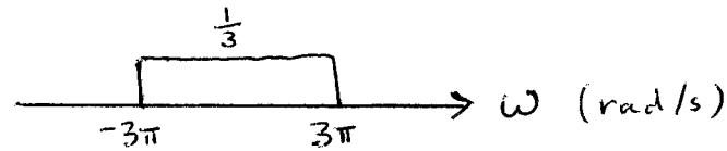
$$\begin{aligned} \Rightarrow H(j\omega) &= \frac{1}{2} \cdot \frac{1}{3} \left\{ u(\omega - 80\pi) - u(\omega - 80\pi - 3\pi) \right\}_{+3\pi} \\ &\quad + \frac{1}{2} \cdot \frac{1}{3} \left\{ u(\omega + 80\pi + 3\pi) - u(\omega + 80\pi - 3\pi) \right\}_{-3\pi} \\ &= \frac{1}{6} \left\{ u(\omega - 77\pi) - u(\omega - 83\pi) \right\} + \frac{1}{6} \left\{ u(\omega + 83\pi) - u(\omega + 77\pi) \right\} \end{aligned}$$
