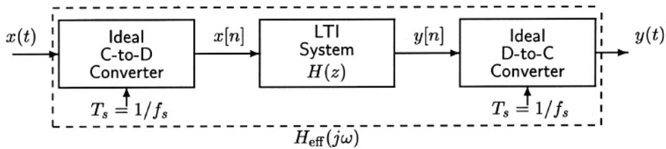
The sampling frequency of the C-D and D-C converters is
