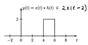
(b) If h(t) = u(t), plot y(t) = x(t) \* h(t) on the graph on the right. Be sure to label the y(t) axis.
