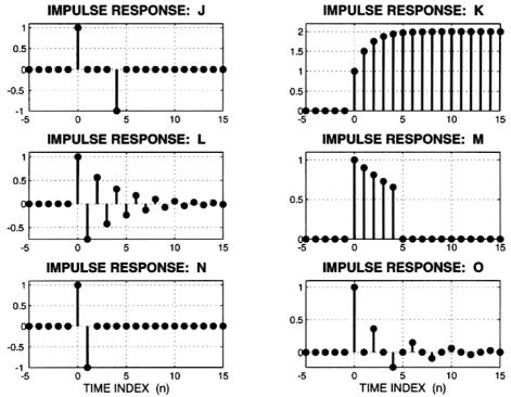
For each of the impulse-response plots (J, K, L, M, N, O), determine which one of the following systems (specified by either an H(z) or a difference equation) matches the impulse response.
