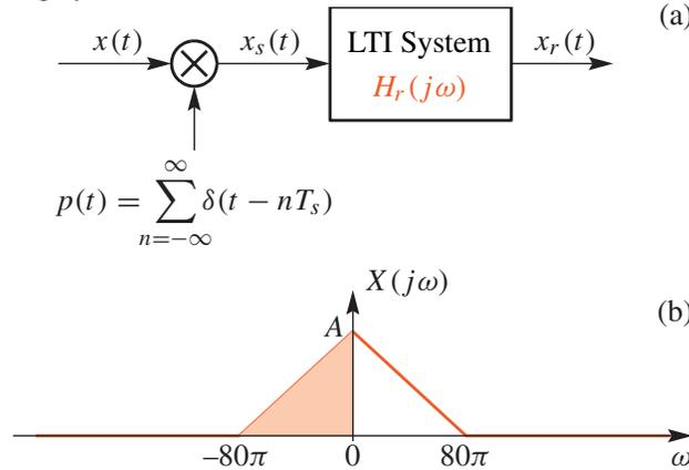
A “typical” bandlimited Fourier transform of the input is also shown above.
