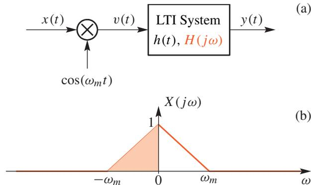
The Fourier transform of the input is also shown above. For all parts below, assume that  $\omega_m = 100\pi$ .
