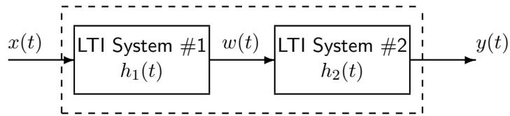
In the cascade of two LTI systems shown in the figure above, the first system has an impulse response
