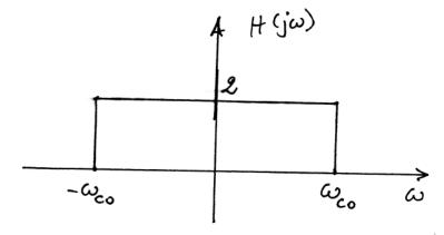
Ideal low-pass filter with gain equal to 2 and  $\omega_m \leq \omega_c \leq 2\omega_c - \omega_m$  (in fact, a mu-ideal low-pass filter will also work).
