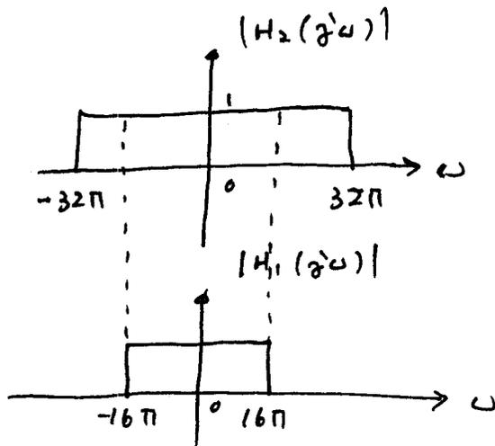
$$\angle H_1(j\omega) = \angle H_2(j\omega) = -3\omega$$
