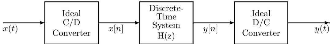
Both the C/D and the D/C run at the same sampling rate, denoted  $T_s$ . The LTI discrete-time system in the middle has the system function
