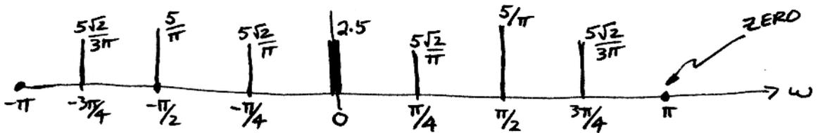
(c) The frequency response of the filter will MULTIPLY the spectrum of the input. Thus the spectrum of the output will be everything EXCEPT the line at DC.
