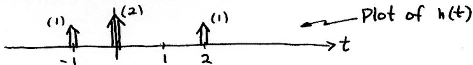
$$\begin{aligned} \text{(b)} \quad H(j\omega) &= \int_{-\infty}^{\infty} h(t) e^{-j\omega t} dt \\ &= \int_{-\infty}^{\infty} \{ \delta(t+1) + 2\delta(t) + \delta(t-2) \} e^{-j\omega t} dt \\ &= \int_{-\infty}^{\infty} \delta(t+1) e^{-j\omega t} dt + \int_{-\infty}^{\infty} 2\delta(t) e^{-j\omega t} dt + \int_{-\infty}^{\infty} \delta(t-2) e^{-j\omega t} dt \end{aligned}$$
