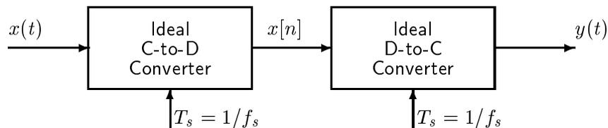
Shown in the figure above is an ideal C-to-D converter that samples  $x(t)$  with a sampling period  $T_s$  to produce the discrete-time signal  $x[n]$ . The ideal D-to-C converter then forms a continuous-time signal  $y(t)$  from the samples  $x[n]$ . Suppose that  $x(t)$  is given by
