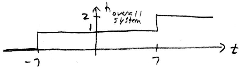
B) Causal if  $h(t) = 0$  for  $t < 0$ . From graph above,  $h(t) \neq 0$  for  $t < 0$ . Therefore, the system is not causal.
