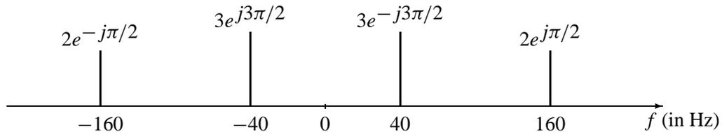
Determine the spectrum for  $x[n]$  when  $f_{si} = 120$  samples/sec. Make a plot for your answer, but label the frequency, amplitude and phase of each spectral component.
