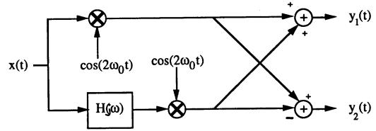
where the frequency response of the system  $H(j\omega)$  and the Fourier transform of x(t) are:
