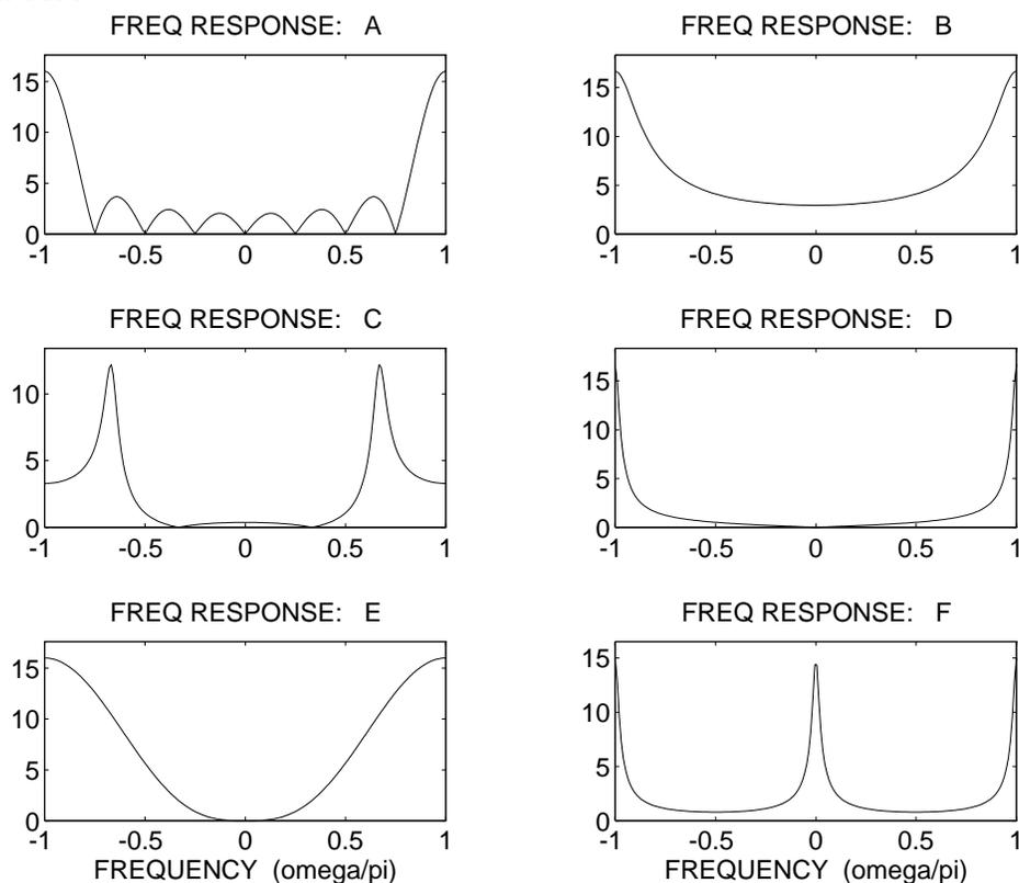
For each of the frequency response plots (A, B, C, D, E, F), determine which one of the following systems (specified by either an  $H(z)$  or a difference equation) matches the frequency response. NOTE: frequency axis is normalized; it is  $\hat{\omega}/\pi$ .
