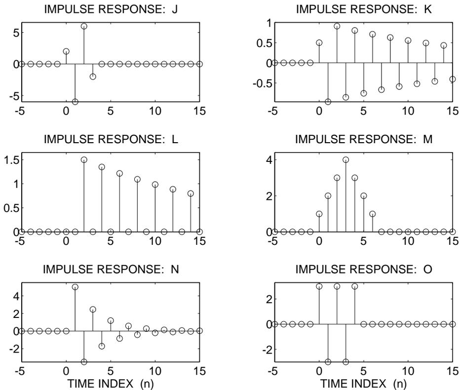
For each of the impulse-response plots (J, K, L, M, N, O), determine which one of the following systems (specified by either an  $H(z)$  or a difference equation) matches the impulse response.
